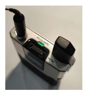
4. To toggle MUTE on and off, simply slide the switch on top of the belt pack. Engaging mute does not disconnect or power down the unit- it simply cuts out the audio.
