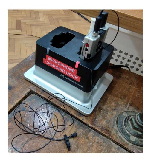
2. The unit should power up automatically and takes a number of seconds to connect to the receiver- the LED on the top of the belt pack should be red during this time. If the LED isn't lit at all you will need to power on the unit manually by pressing and holding the red power button on the side of the unit.
