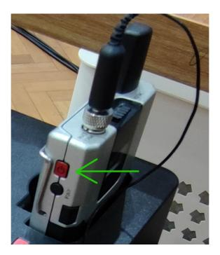
3. When connected the LED should change to either green or yellow. If green, the microphone is on and is un-muted. You should be able to hear your voice amplified in the lecture room when you speak into it. If the LED is yellow it means that the MUTE switch is engaged.
