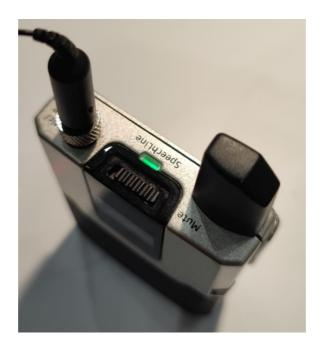
4. To toggle MUTE on and off, simply slide the switch on top of the belt pack. Engaging mute does not disconnect or power down the unit- it simply cuts out the audio.
