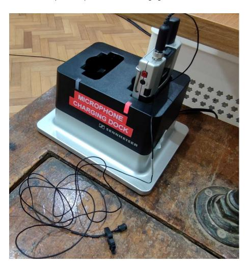
2. The unit should power up automatically and takes a number of seconds to connect to the receiver- the LED on the top of the belt pack should be red during this time. If the LED isn't lit at all you will need to power on the unit manually by pressing and holding the red power button on the side of the unit.
